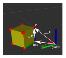
• to transform  $_{box}P_2$  into the global frame  $_{global}P_2$ , multiply with  $_{global}T_{box}$
