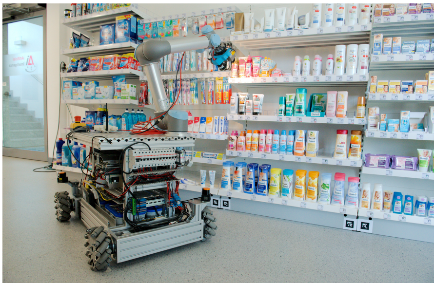
Figure 1.2: Donbot robot in action at the supermarket setup [11]
