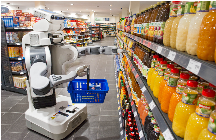
Figure 1.1: Robots deployed in super market to pick and place grocery items [11]
